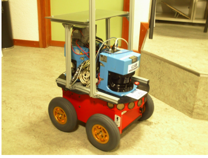
Figure 14: Pioneer 3-AT robot equipped with two laser range scanners.
