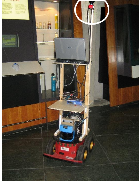
Fig. 1. The vision system in the tour-guide mobile robot, based on a Pioneer 2-AT, placed at the Domus Museum in A Coruña (Spain). The omnivision camera is marked with a circle.
