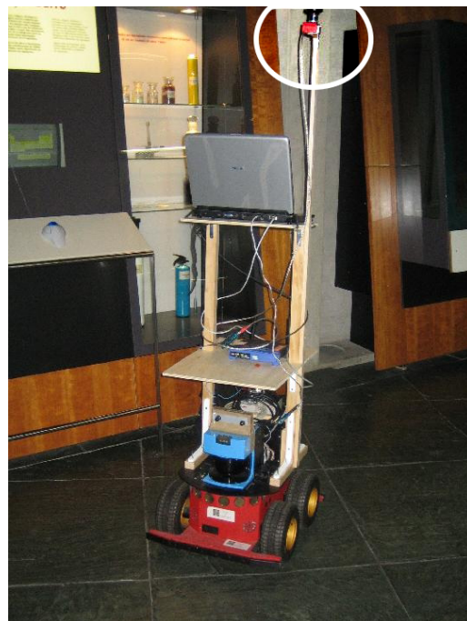
Fig. 1. The vision system in the Guide Mobile Robot, based on Pioneer IIAT, used at the Domus Museum in A Coruña (Spain). The omnivision camera is marked with a circle.
