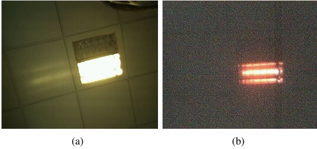
Fig. 5. Optical filtering effect: (a) original image, (b) filtered image (only IR light is detected).
