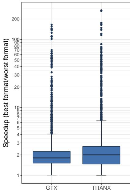
Fig. 5: Speedup obtained considering the best storage format with respect to the worst one for all the matrices in the dataset.
