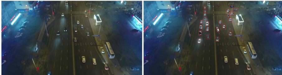
Figure 1: We describe a pipeline for small object data augmentation able to populate an original frame (left) with new generated small objects (right), highlighted in red.
